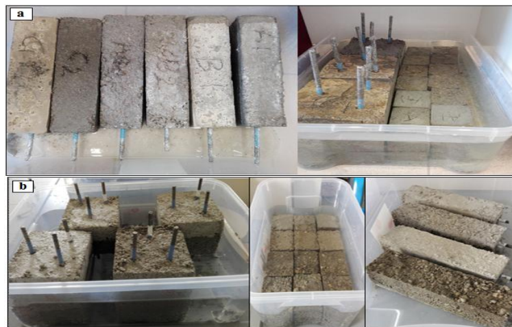
Figure 3 Specimens of half-cell corrosion potential test and linear polarization resistance test immersed partially and specimens of chloride ion ingress test completely immersed in 3.5% NaCl solution a) samples with green inhibitor, b) with calcium nitrate
